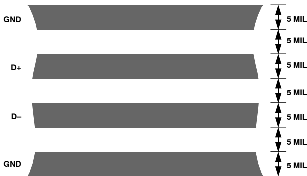
Figure 22. Typical Arrangement of Signal Tracks
