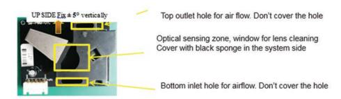
The heater resister is installed inside of dust sensor for inducing the forced air convection and the heated air flows from bottom side to top side direction. The heater resister's temperature is increased over  $40^{\circ}$ C than atmosphere. So, vertical positioning of dust sensor is important for air flow direction and speed optical zone. The air flow direction and flow speed can affect the signal output of dust sensor. Please keep  $\pm$  5 degree position vertically.
