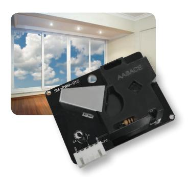
SM-PWM-01C dust sensor detects dust particle concentration in air by using an optical sensing method. An infrared light emitting diode (IR LED) and a photo-sensor are optically arranged in the device. The photosensor detects the reflected IR LED light by dust particles in air. The dust sensor can detect the small particles like cigarette smoke and can distinguish small particles like smoke from large house dust by the pulse pattern of the signal output.
