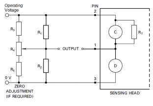
$\begin{array}{ll} R_1 = R_2 = 500\Omega \text{ to } 10 \text{ k}\Omega \\ R_3 = R_5 \simeq 10R_1 \\ R_4 \simeq 20R_1 \end{array}$
