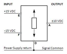
A through F: Connector pin assignments
