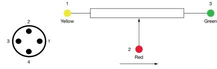
Direction of wiper displacement with shaft extended
