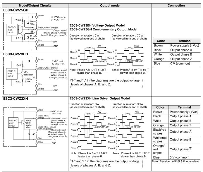
Note: 1. The shielded cable outer core (shield) is not connected to the inner area or to the case.
